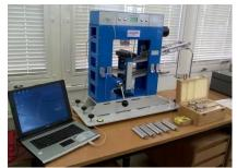
Figure 2. Cut resistance testing device in the laboratory of INNOVATEXT
