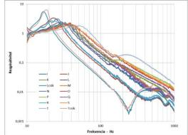
Figure 4. Vibration isolation of the measured samples
